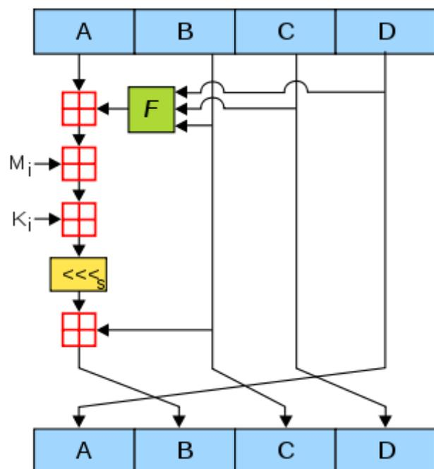
Figure 1. One MD5 operation. MD5 consists of 64 of these operations, grouped in four rounds of 16 operations.  $F$  is a nonlinear function; one function is used in each round.  $M_i$  denotes a 32-bit block of the message input, and  $K_i$  denotes a 32-bit constant, different for each operation.  $\lll_s$  denotes a left bit rotation by  $s$  places;  $s$  varies for each operation.  $\boxplus$  denotes addition modulo  $2^{32}$ .
